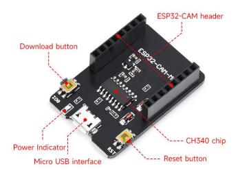
The ESP32-CAM-MB programmer is a shield that you attach to your ESP32-CAM board GPIOs. The programmer comes with the CH340C USB to serial chip. This allows you to program the ESP32-CAM using the USB port on the shield. The shield also comes with a RESET button. This may be useful to easily reset the ESP32-CAM or put it into flashing mode.
